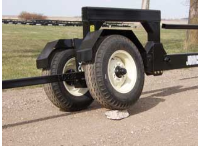
Each wheel oscillates independently.
